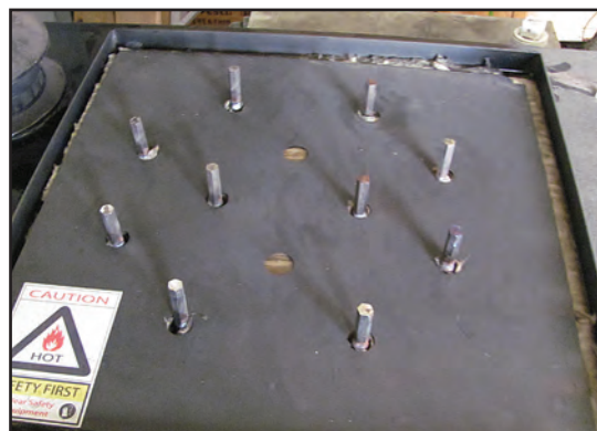
Figure 12 - Heat exchanger tube brush ends
