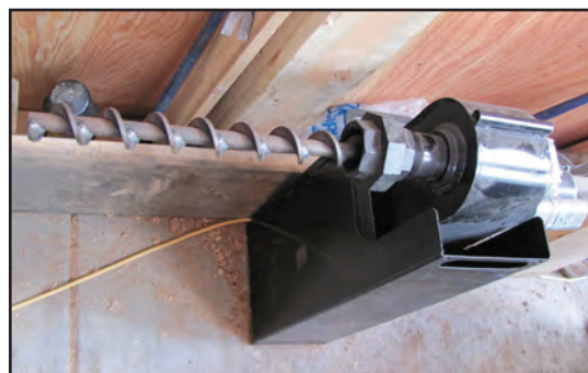
Figure 11 - Ash removal auger
